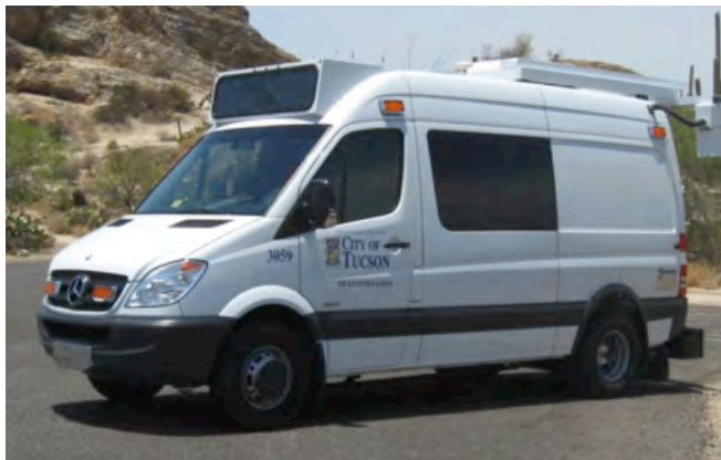
City of Tucson's Automated Road Analyzer (ARAN) van is used to collect pavement condition data for the entire region.
