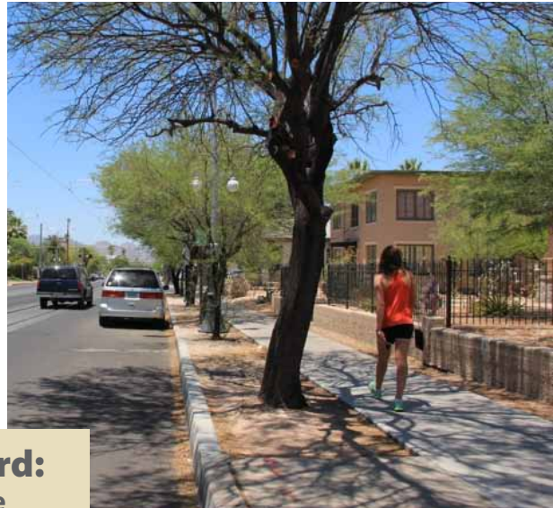
Residential sidewalk. A 5-foot sidewalk and 5-foot planting strip provide adequate walking space and room to plant shade trees.
