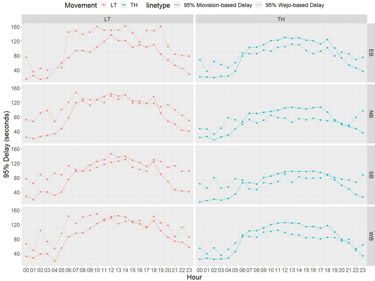
Figure 4-25. Comparison between Miovison and Wejo-based 95<sup>th</sup> percentile delay at La Cholla Blvd. / River Rd.
