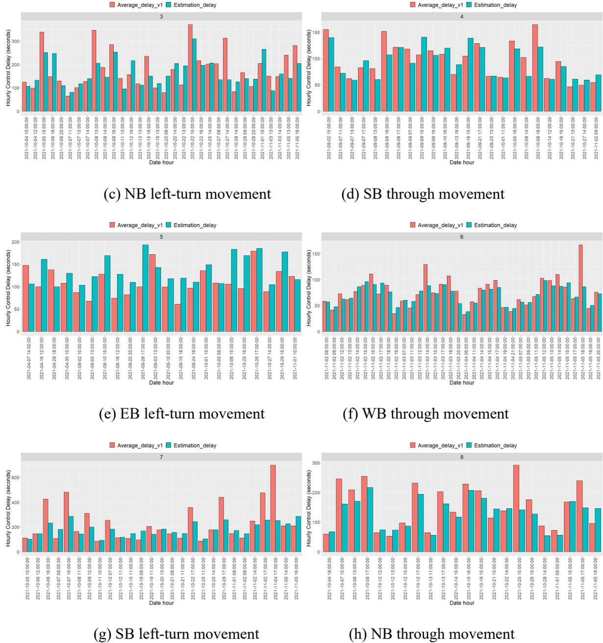
Figure 6-9. Ground-truth and estimated control delay comparison at Speedway Blvd. & Euclid Ave.
